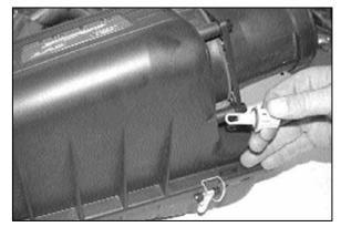
23. Remove the temp sensor from the factory air box as shown.
