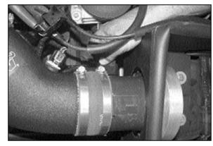
29. Reconnect the mass air sensor electrical connection as shown.
