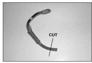
19. Cut the end off the idle air vent tube just below bead as shown. Then re-install vent tube back onto vehicle.
