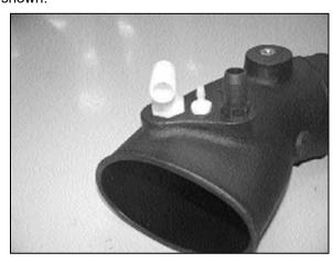
16. Install the provided vent fitting onto the new K&N® intake tube as shown.
