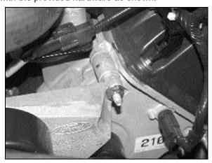
13. Remove the 8mm nut from stud that retains the idler pully bracket.
