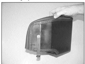
11. Install the "L" bracket onto heat shield as with the provided hardware as shown.
