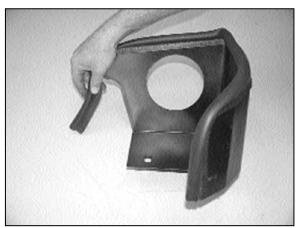
9. Install edge trim onto the heat shield as shown. Trim if needed.
